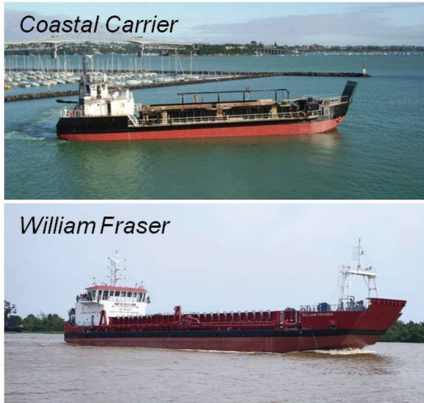
Figure 9: Photographs of the two trail-suction hopper dredgers (TSHDs) used by MBL. The Coastal Carrier was decommissioned October 2019 and the William Fraser has replaced it.
